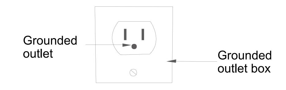
WARNING: Risk of electric shock. Connect the unit only to a circuit protected by a ground-fault circuit-interrupter (GFCI).
