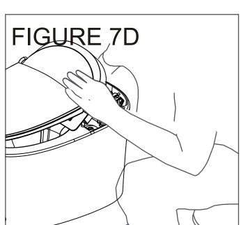
Caution: Do not move the toilet bowl around once the toilet bowl is in position. It can damage the wax ring seal and result in water leakage.
