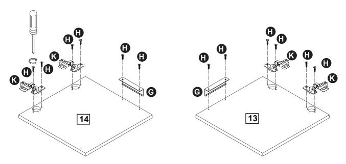
Attach (2) Handles (Part G) using (4) 3.5\*14mm Screws (Part H).
