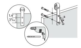
The rubber ends are used to protect the door from touching the rail when sliding the door. You need to drill holes on the door top side , please drill the holes 1/2 away from the edge of the door. Then install the rubber ends on the door.
