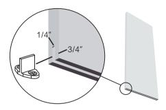
Install the hangers onto the door according to the measurement in the pictures below.
