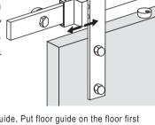
Install the floor guide. Put floor guide on the floor first to fix a suitable position and make a mark so that the tip of the floor guide can work well in the slot.
