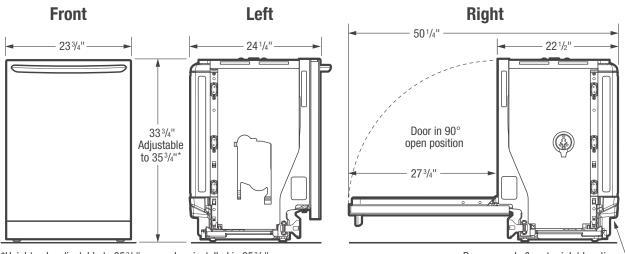
\*Height only adjustable to 35<sup>3</sup>/<sub>4</sub>" max. when installed in 35<sup>3</sup>/<sub>4</sub>" max. standard cabinetry cutout. (Dimensions do NOT include insulation – insulation blanket may be compressed during installation.)
