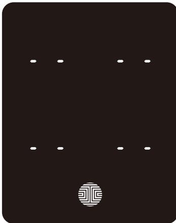
If there are no **Access Codes** registered in your smart lock, **Check Access Code** mode will be invalid. The default **Access Code** will not be shown on the display keypad, and you will see the following screen shown to the left instead.
