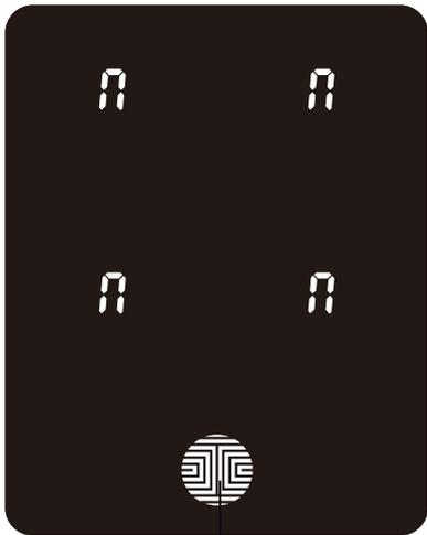
If the two (2) **Access Codes** you entered does not match, an error message will appear on the screen (As shown to the left). Press **OK** to return to the **Programming Screen** and try again. See **Section 3.3**
