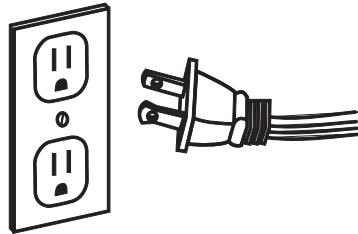
**⚠ WARNING:** It is normal for the power cord to feel warm to the touch. However, a loose fit between the outlet and the plug may cause overheating of the plug. If this occurs, try inserting the plug into a different outlet. Contact a qualified electrician to inspect the original outlet for damage.
