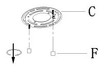
6. Attach the mounting plate (C) to outlet box with the mounting screws (B).
