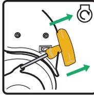
9. For electric start only-Flip the engine switch to the START (II) position for a few seconds and then release.
