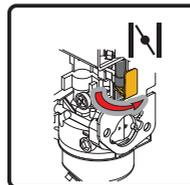
8. For recoil start only-Pull the starter cord slowly until resistance is felt and then pull rapidly.
