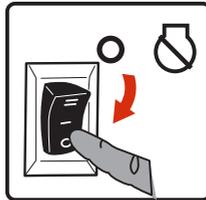
4. Flip the battery switch to **"OFF" (O)** position.
