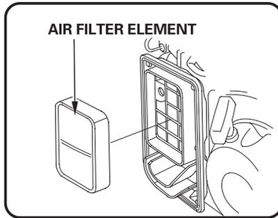
(b) Saturate foam air filter element with clean engine oil and squeeze in a clean cloth to remove excess oil.
