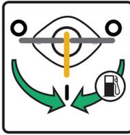
5. Flip the engine switch to the "RUN"(I) position.
