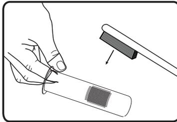
4. Replace the spark arrester if it is damaged. If replacement parts are required, make sure to use only FIRMEN original equipment replacement parts.
