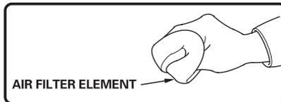
(c) Reinstall clean or new air filter element.
