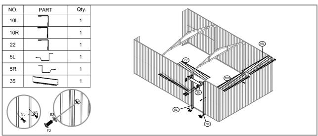
The below assembly is for the front door & roof , pls ignore the side door direction in the assembly picture.
