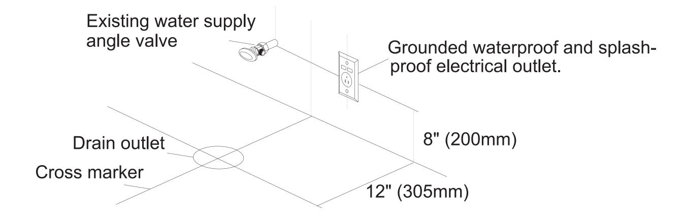
(2) Installation of floor flange.
