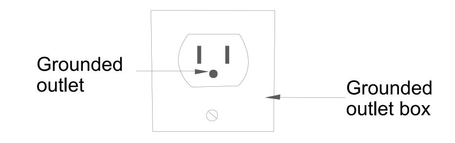
\*WARNING: Risk of electric shock Connect only to a circuit that is protected by a ground-fault circuit-interrupter (GFCI).
