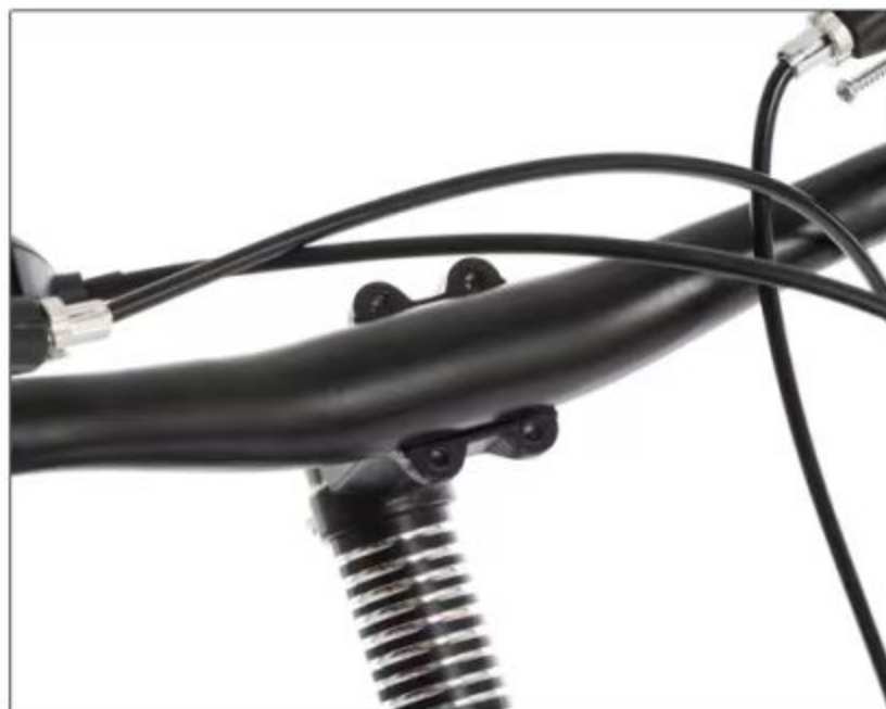
8. Install the front handlebar
