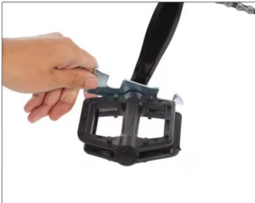
16. Install the left side counterclockwise and tighten it
