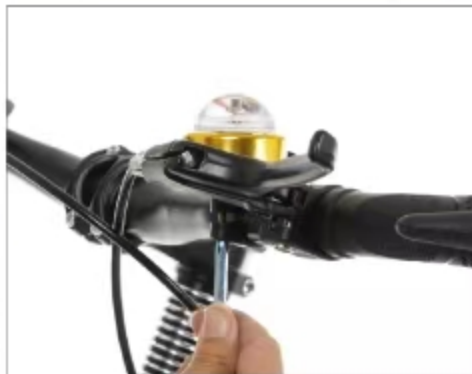
23. Install the car bell onto the handlebar
