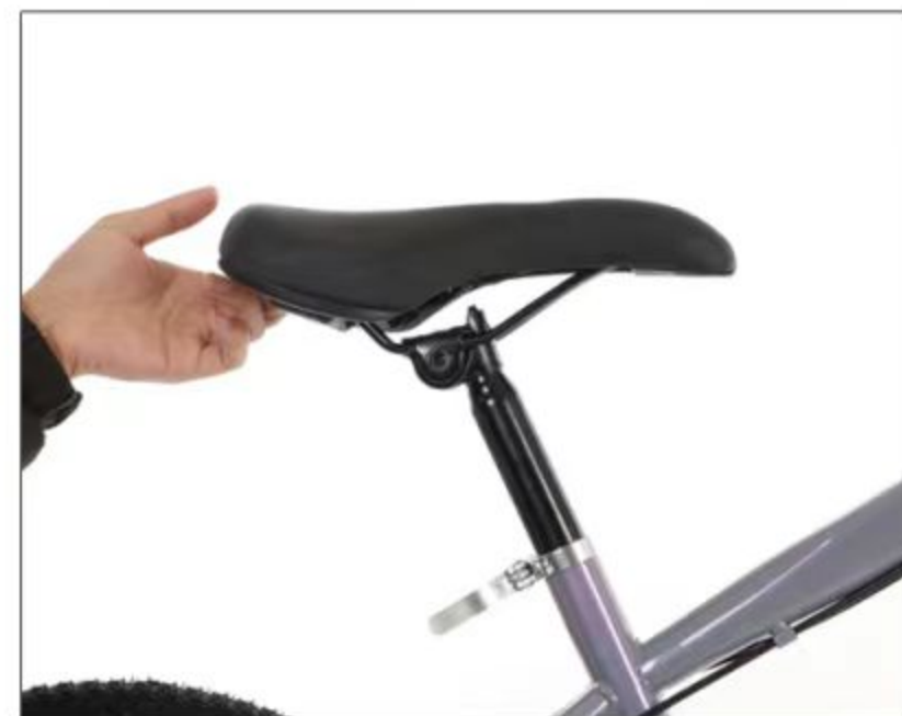
12. Install the seat into the frame
