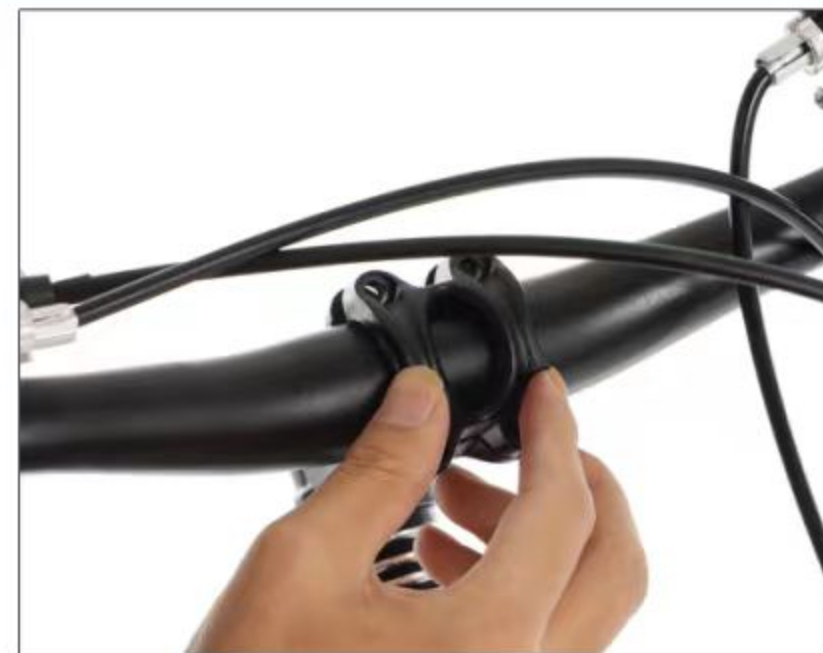
9. Buckle up the vertical buckle cover
