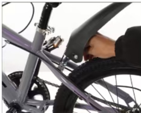
20. Install the rear mudguard
