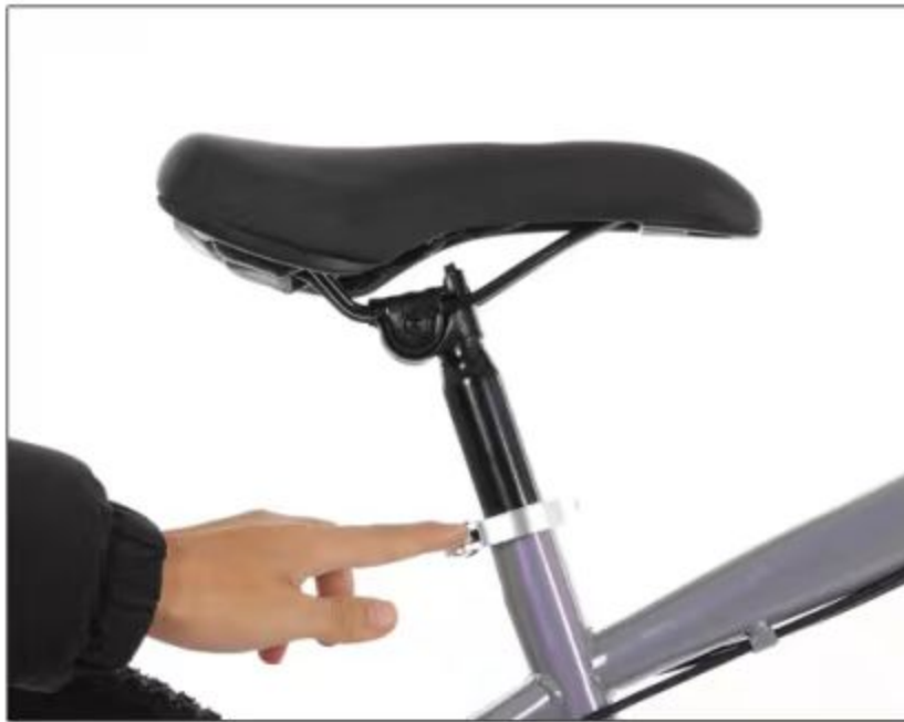
13. Tighten the seat and quickly remove it
