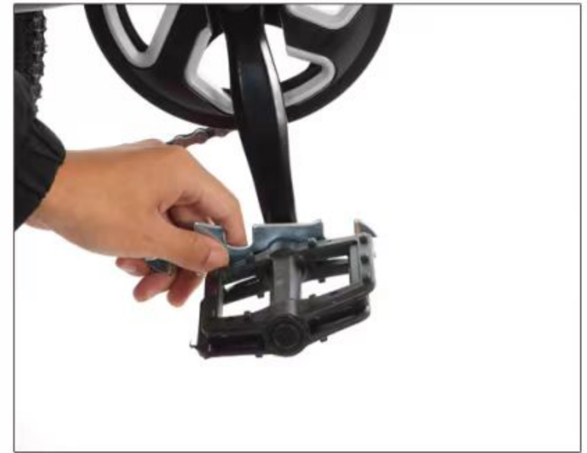
15. Install R and tighten clockwise on the right side
