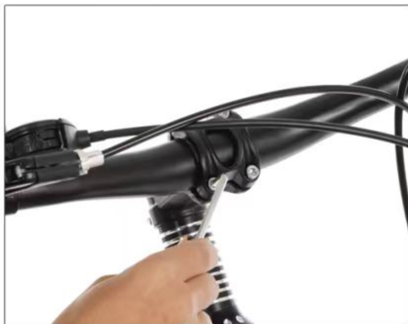
10. Tighten the screws to secure firmly
