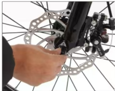
24. Install the waterproof cap
