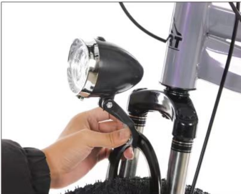
17. Screw through the front fork
