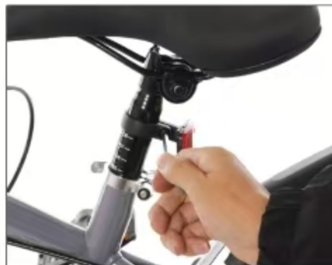
21. Install the rear taillights onto the seat tube
