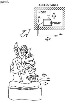
**3.** Fill the reservoir with water, ensuring the pump is completely submerged during operation; approximately 2 gallons.
