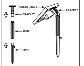
**5.** Insert the spike into the ground. Position the solar panel to face south (in the northern hemisphere) to make the most of daylight hours. It is important to angle the solar panel towards the sun when the sun is at its highest point. Ensure trees, shrubs, or buildings do not shade the solar panel.
