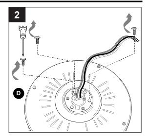
3. Pull wires up through hole in the middle of the canopy (B) and attach canopy (B) to motor housing (D) using the three screws previously removed.
