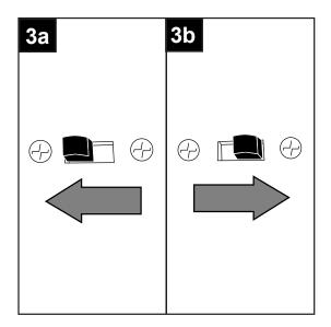
3c. **IMPORTANT:** Reverse switch must be set either *completely* LEFT or *completely* RIGHT for fan to function. If the reverse switch is set in the middle position, fan will not operate.
