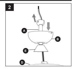
3. Slip downrod (A) into yoke, align holes and re-install pin (L) and clip (M). Tighten set screws and then tighten nuts on the set screws. Slide yoke cover (E) down until it rests on top of motor housing (D).
