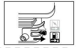
Move the Choke to the OPEN **Position**
