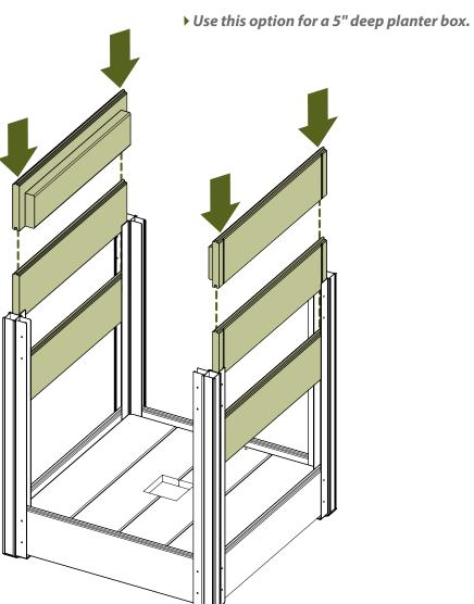
Top support boards **(C)** should be on the opposite 2 sides as the bottom support boards.
