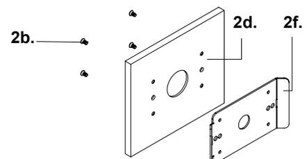
\*For Single Gang Box Installation, the backplate (2f) can be detached from the cover plate (2d) by removing the cover plate screws (2b).
