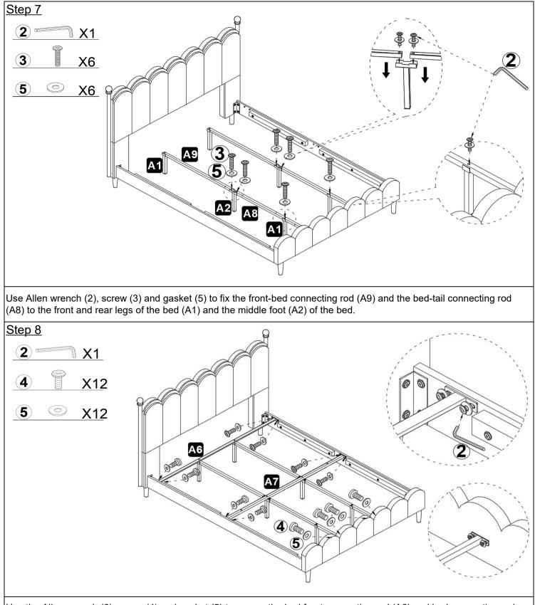
Use the Allen wrench (2), screw (4) and gasket (5) to secure the bed front connecting rod (A6) and bed connecting rod (A7) to the bed side plate (B3&).
