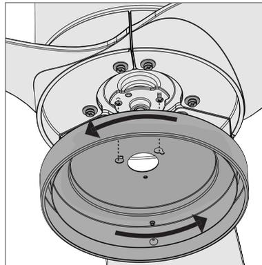
Feed the wire plugs through the center hole of the upper switch housing, then wrap keyhole slots around the screws and twist counterclockwise.
