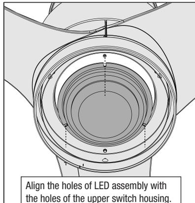
Align the holes of LED assembly with the holes of the upper switch housing. Make sure all the wires from the fan and the light kit are snug inside the center of the light kit, not pinched in between the upper switch housing and the light kit or hanging out of the sides.
