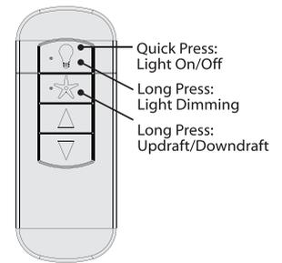
Quickly press the Light button to turn the lights off and on. Hold the Light button to raise and dim the light level.
