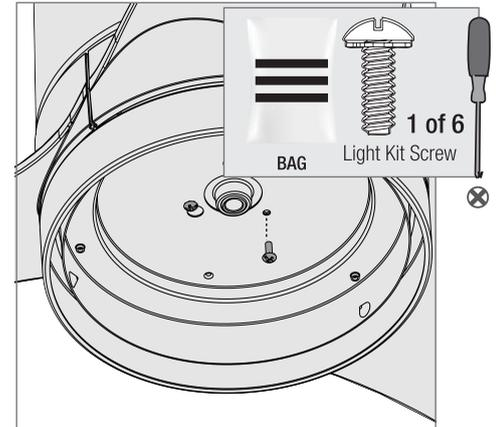
Insert the third screw, found in the ≡ hardware bag, into place and then tighten all three screws.
