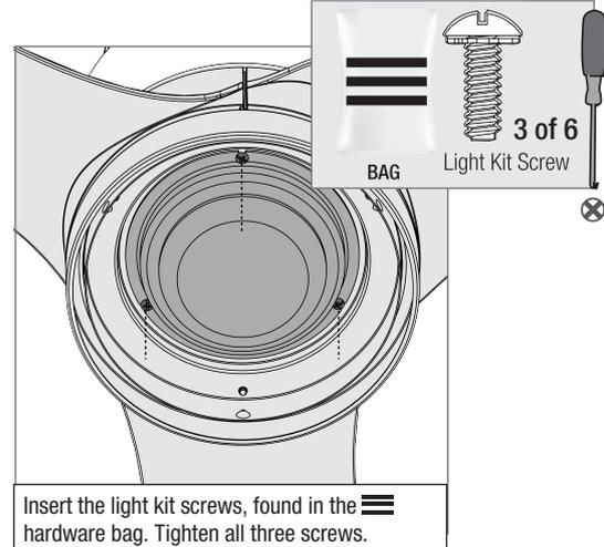
Insert the light kit screws, found in the ≡ hardware bag. Tighten all three screws.
