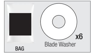
Put the blade washers found in the ■ hardware bag onto the blade screws found in the X hardware bag. Then install the blade screws to secure each blade to the fan.
