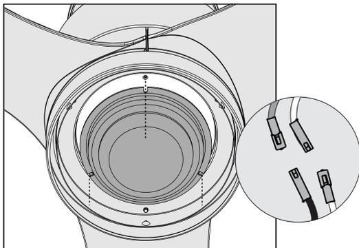
Connect the singlepin connectors to the connectors from the fan. Connect the white wires together. Connect the blue and black wires together.
