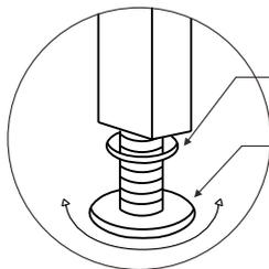
2.Adjust screw nut to the level position
