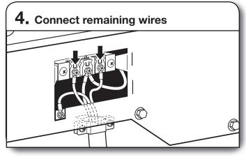
Connect remaining wires to outer terminal block screws. Tighten screws. Finally, reinsert tab of terminal block cover into slot of dryer rear panel. Secure cover with hold-down screw. Now, go to "Venting Requirements."
