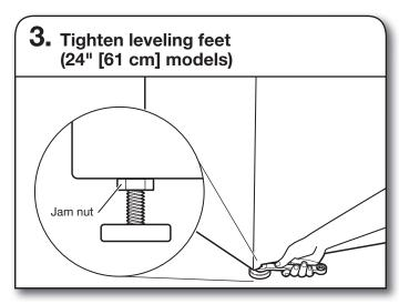
When washer/dryer is level, use a 9/16" or 14 mm open-end or adjustable wrench to turn jam nuts counterclockwise on leveling feet tightly against washer/dryer cabinet.
