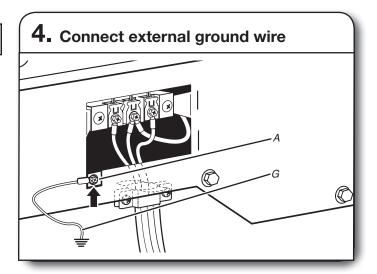
Connect a separate copper ground wire (G) from the external ground conductor screw (A) to an adequate ground. Finally, reinsert tab of terminal block cover into slot of dryer rear panel. Secure cover with hold-down screw. Now, go to "Venting Requirements."
