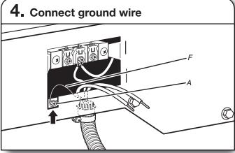
Connect ground wire (green or bare) (F) of direct wire cable to external ground conductor screw (A). Tighten screw.
