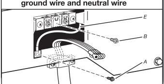
Remove center terminal block screw (B). Remove neutral ground wire (E) from external ground conductor screw (A).
