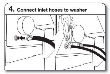
Attach hot water hose to the right-hand (red) inlet valve. Screw coupling by hand until it is snug. Use pliers to tighten couplings an additional two-thirds turn. Repeat with cold water inlet valve (left-hand [blue] inlet valve).
