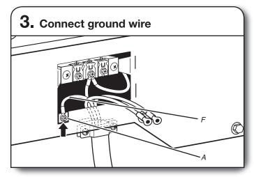
Connect ground wire (F) (green or bare) of power supply cord to external ground conductor screw (A). Tighten screw.
