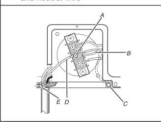
Remove center terminal block screw. Remove neutral ground wire from external ground conductor screw. Connect neutral ground wire and the neutral wire (white or center wire) of power supply cord under center terminal block screw. Tighten screw.
