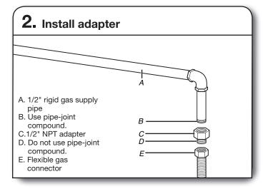
Install the adapter on the 1/2" rigid gas supply pipe using pipe-joint compound.
