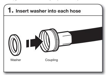
Insert a new flat washer into each end of the inlet hoses (not provided). Firmly seat the washers in the couplings.
