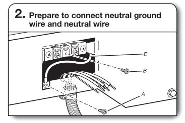
Remove center terminal block screw (B). Remove neutral ground wire (E) from external ground conductor screw (A).
