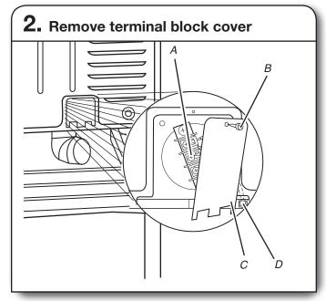
Before you start, disconnect power. Remove hold-down screw (B) and terminal block cover (C).
