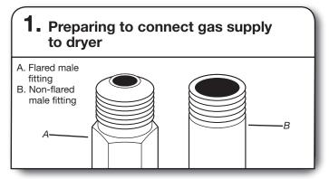
Remove red cap from flexible gas connector. Remove the 1/2" NPT adapter from the flexible gas connector (it will be necessary to use two adjustable wrenches). Use pipe-joint compound on threads of all non-flared male fittings. If flexible metal tubing is used, be sure there are no kinks.
