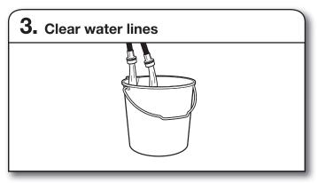
Run water for a few seconds through hoses into a laundry tub, drainpipe, or bucket to prevent clogs. Water should run until clear.
