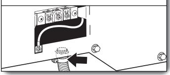
Put direct wire cable through the strain relief. The strain relief should have a tight fit with the dryer cabinet and be in a horizontal position. Tighten strain relief screw against the direct wire cable.
