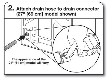
Open clamp. Twist hose back and forth while pushing onto drain connector at the lower left (27" [69 cm] models) or lower center (24" [61 cm] models) portion of the rear of the washer/dryer. Continue until hose contacts the ribbed stops on the cabinet. On 27" (69 cm) models, place clamp over the area on the hose marked "CLAMP." On 24" (61 cm) models, place clamp over the smooth area on the hose between the two ribs. Release clamp.
