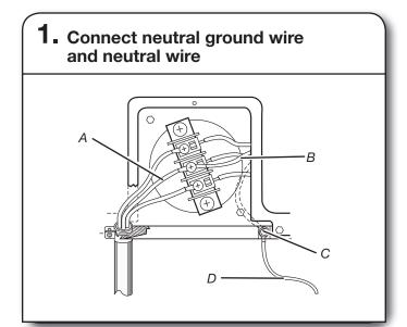
Remove center terminal block screw. Remove neutral ground wire from external ground conductor screw. Connect neutral ground wire and the neutral wire (white or center wire) of power supply cord under center terminal block screw. Tighten screw.
