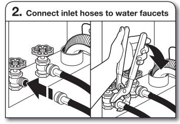
Attach hose to hot water faucet. Screw on coupling by hand until it is seated on washer. Use pliers to tighten couplings an additional two-thirds turn. Repeat this step with second hose for cold water faucet.
