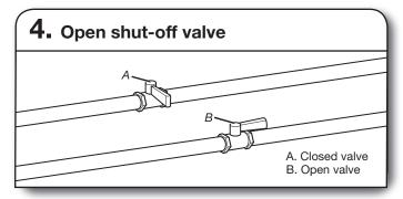
Open shut-off valve in supply line; valve is open when handle is parallel to gas pipe. Then, test all connections by brushing on an approved noncorrosive leak-detection solution. Bubbles will show a leak. Correct any leak found.
