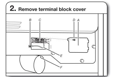
Before you start, disconnect power. Remove hold-down screw (D) and terminal block cover (A).
