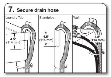
Secure drain hose to laundry tub leg, drain standpipe, or inlet hoses for wall standpipe with plastic strap included in the parts package.
