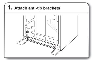
**IMPORTANT:** The anti-tip brackets must be installed on 27" (69 cm) models to avoid possible tipping backward of the washer/dryer.
