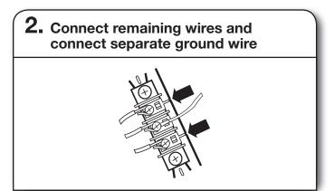
Connect the other wires to outer terminal block screws. Tighten screws. Tighten strain relief screws. Connect a separate copper ground wire from the external ground conductor screw to an adequate ground. Insert tab of terminal block cover into slot of dryer rear panel. Secure cover with hold-down screw. Now go to "Venting Requirements."
