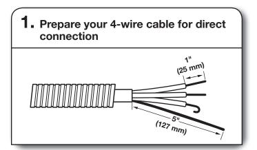
Direct wire cable must have 5 ft. (1.52 m) of extra length so washer/dryer may be moved if needed.
