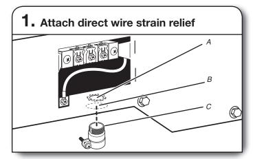
Unscrew the removable conduit connector (A) and any screws from a 3/4" (19 mm) UL Listed strain relief. Put the threaded section of the strain relief (C) through the hole below the terminal block opening (B). Reaching inside the terminal block opening, screw the removable conduit connector (A) onto the strain relief threads.
