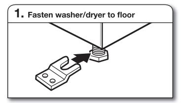
For mobile home use: Washer/dryers with gas dryers must be securely fastened to the floor.
