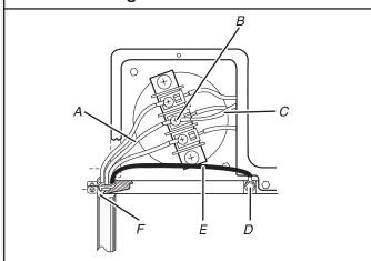
Connect ground wire (green or bare) of power supply cord to external ground conductor screw. Tighten screw.
