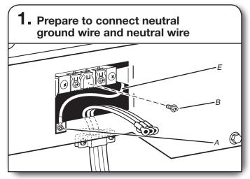
Remove center terminal block screw (B). Remove neutral ground wire (E) from external ground conductor screw (A).
