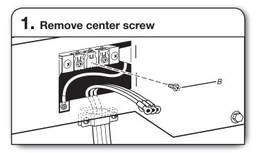
Remove center terminal block screw (B).
