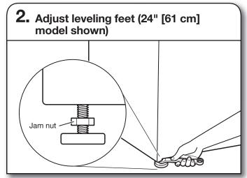
If washer/dryer is not level, prop up front of washer/dryer about 4" (102 mm) with a wood block or similar object that will support weight of washer/dryer.
