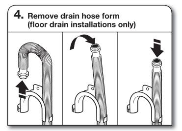
For floor drain installations, you will need to remove the drain hose form from the end of the drain hose. You may need additional parts with separate directions. See "Tools and Parts."
