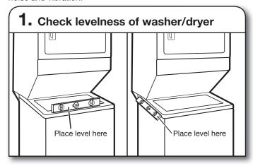
With washer/dryer in its final location, place a level on top edges of washer/dryer. Use side seam as a guide to check levelness of sides. Check levelness of front using lid, as shown. Rock washer/dryer back and forth to make sure all four feet make solid contact with floor. If washer/dryer is level, skip to step 3 (24" [61 cm] models) or "Install Anti-Tip Brackets" (27" [69 cm] models).
