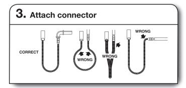
Attach the flexible gas connector to the 1/2" NPT adapter. Do not use pipe-joint compound for this connection.
