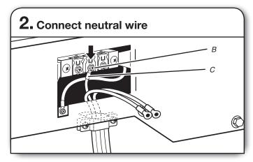
Connect neutral wire (white or center) (C) of power supply cord to center terminal block screw (B). Tighten screw.
