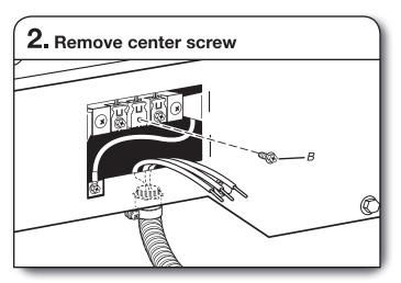
Remove center terminal block screw (B).
