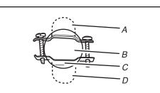
Remove the screws from a 3/4" (19 mm) UL Listed strain relief. Put the tabs of the two clamp sections (C) into the hole below the terminal block opening (B) so that one tab is pointing up (A) and the other is pointing down (D), and hold in place. Tighten strain relief screws just enough to hold the two clamp sections (C) together.
