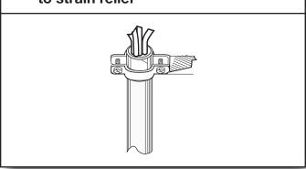
Put power supply cord through the strain relief. Be sure that the wire insulation on the power supply cord is inside the strain relief. The strain relief should have a tight fit with the dryer cabinet and be in a horizontal position. Do not further tighten strain relief screws at this point.
