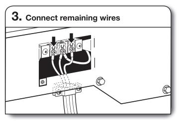
Place remaining wires under outer terminal block screws (hooks facing right). Tighten screws.
