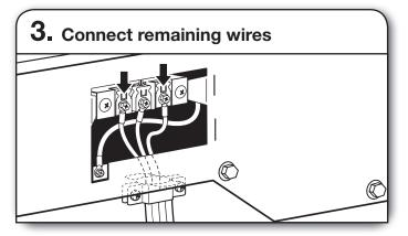
Connect remaining wires to outer terminal block screws. Tighten screws. Finally, reinsert tab of terminal block cover into slot of dryer rear panel. Secure cover with hold-down screw. Now, go to "Venting Requirements."
