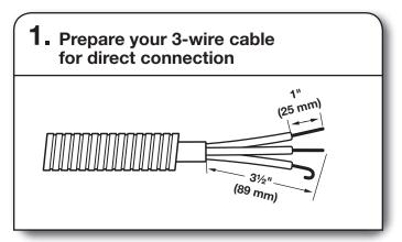
Direct wire cable must have 5 ft. (1.52 m) of extra length so washer/dryer may be moved if needed.
