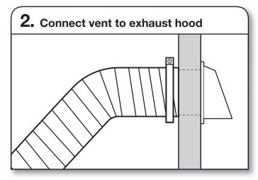
Vent must fit inside the exhaust hood. Secure vent to exhaust hood with 4" (102 mm) clamp. Run vent to dryer location using straightest path possible. Avoid 90° turns. Use clamps to seal all joints. Do not use duct tape, screws, or other fastening devices that extend into interior of vent to secure vent, because they can catch lint.
