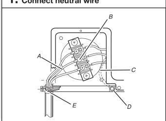
Loosen or remove center terminal block screw. Connect neutral wire (white or center wire) of power supply cord to the center terminal screw of the terminal block. Tighten screw.
