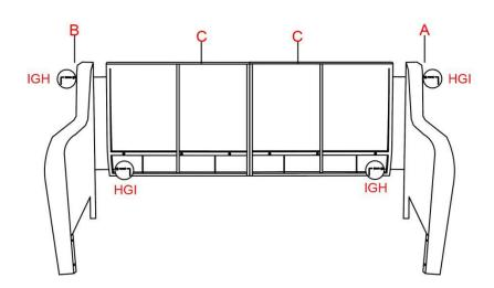
3. Secure assembled front apron (E) to chair arms (A&B) with 4 washers (H) and 4 screws (J) by using allen wrench (I). Do not tighten all screws now.
