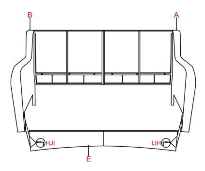
4. Secure seat panel (D) to assembled chair back (C) and assembled front apron (E) with 12 washers (H) and 12 screws (L) by using allen wrench (I). Do not tighten all screws now.
