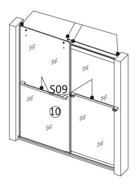
Put the waterproof seal strips on the panel Secure the towel bars on the glass
