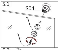
Secure the rollers on the glass Put the roller on the rail track
