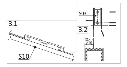
Step 4. Put the the bracket cover on and secure it by screws
