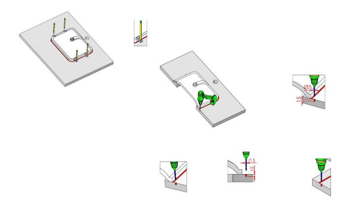
If installing in wood countertop, use #10 wood screw for installation of the mounting bracket.
