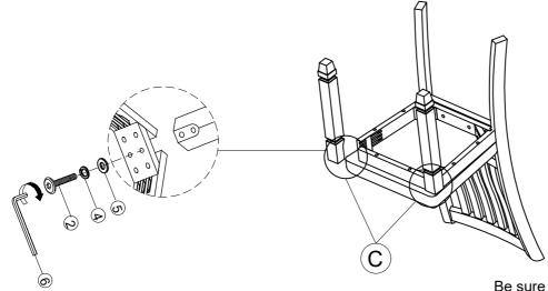
Be sure the legs are level then fully tighten the leg bolts!
