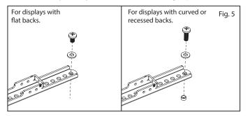
**2** Determine the correct diameter of screw to use by carefully trying one of each size (M4, M5, M6 and M8) from the hardware kit. Do not force any of the screws - if you feel resistance stop immediately and try a smaller diameter screw.
