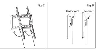
**IMPORTANT!** Verify that both arms are locked to the wall plate. For safety reasons, this mount cannot be used unless both arms are securely locked (see Fig. 8).
