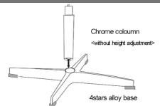
Place the column onto the base
