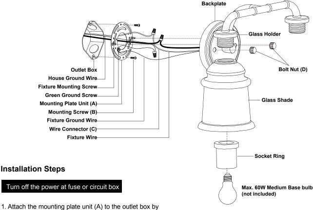
using two mounting screws (B).
