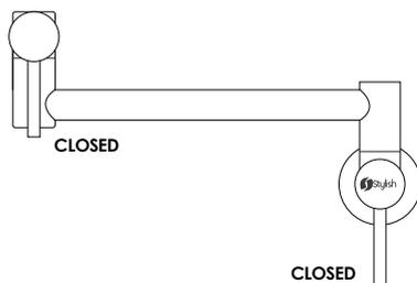
With both pot-filler handles in close position, open water supply.
