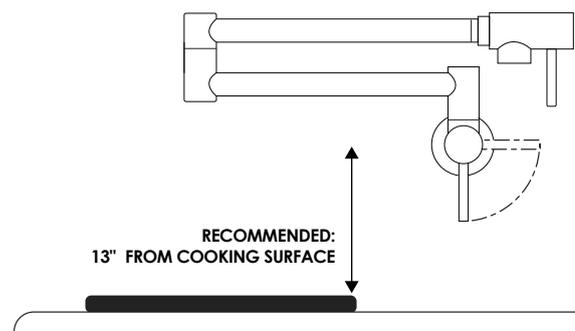
Prior to installation, rough in plumbing must be completed. The position of your potfiller should be considered prior to starting. When fully extended from wall, the reach of the potfiller is 21 inches. Use a position on wall that allows potfiller to reach furthest cooking position for filling (Fig. 1). We recommend aligning the potfiller valve to either left or right side of the cooking surface. Access to valve should not be over the center of the cooking area.
