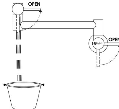
Confirm pot-filler operation, check for any leak.
