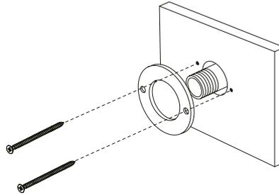
Secure decorative plate on wall, be careful no to interfere with installed pipe.
