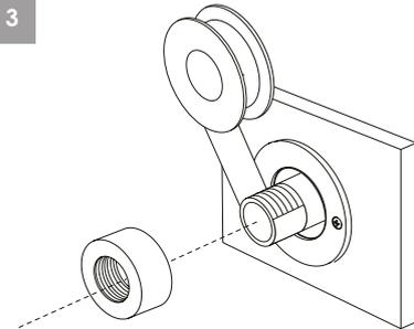
Thread the adjustable ring up to the decorative plate and then wrap with Teflon the pipe thread area exposed.
