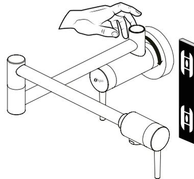
This pot-filler has an adjustable ring at the base that is used to tighten the pot-filler, adjust the ring until pot filler is firmly positioned.
