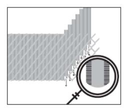
Simply insert slats into the chain link fence with rounded edge FACING DOWN and push downward.
