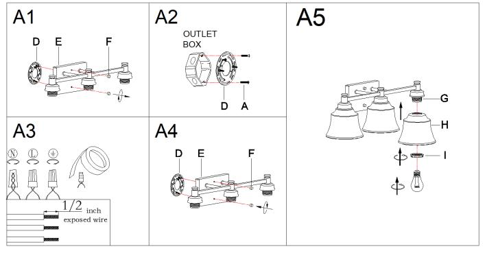
Connect wires according to the below chart
