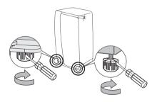
When installing the refrigerator, make sure both legs contact the floor for secure installation.
