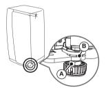
Open the door that needs to be adjusted and loosen the clamping nut (A) at the bottom of the door by turning it clockwise ( ) using the spanner included in the product package. (Raise the lower of the two doors first.)
