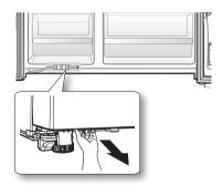
Remove the two water lines (White for water and the other for ice) by pressing the coupler (1) and pulling the water line (2) away.
