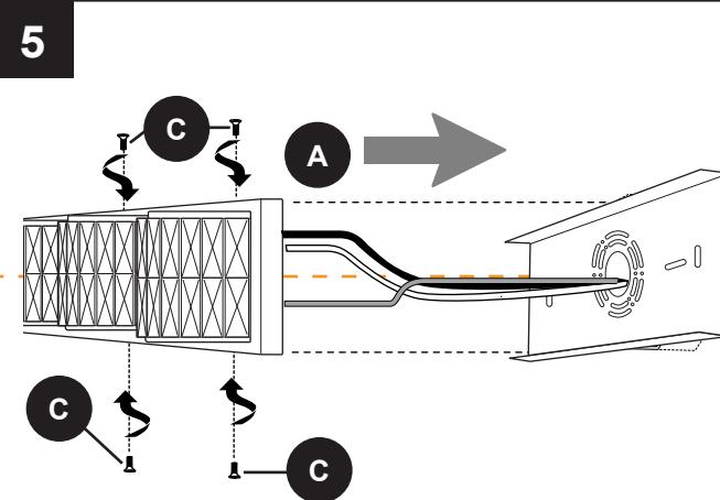
Before tightening C completely, use level (not included) to check A -- adjust if necessary.
