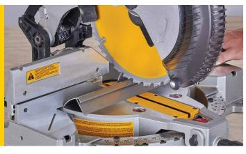
Measure and cut Vinyl Plank Stair Nosing to needed length using either a miter saw, chop saw or hacksaw with the highest number of teeth per inch.
