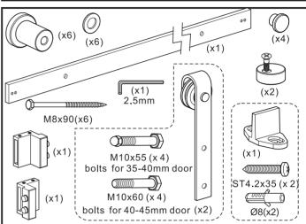
To obtain the maximum weight capacity, all rail mounting fasteners must be mounted directly into solid wood. Do NOT install directly onto a drywall surface. A solid wood header is recommended as shown in instruction box 2.
