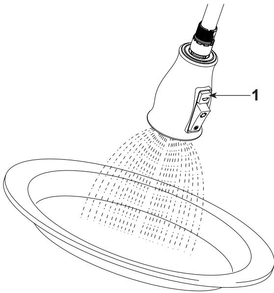
**A.** Sprayer will lock into position when brought into proximity of the spout magnet. The sprayer can be removed by either pulling directly out from the spout or by twisting 90° in either direction which will cause the magnets to repel and the head to decouple from the spout (recommended).
