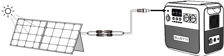
**Warning:** The open circuit voltage of solar panels cannot exceed 60V, otherwise it will damage the device.
