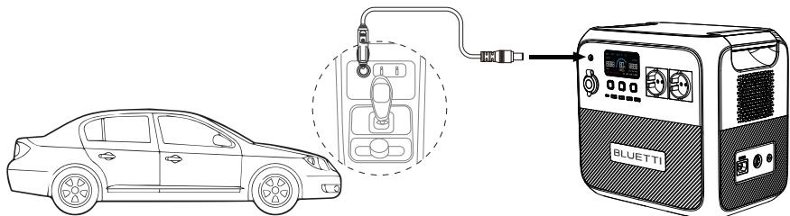
**Warning:** Cigarette lighter MUST be fully inserted into the lighter port of the machine.
