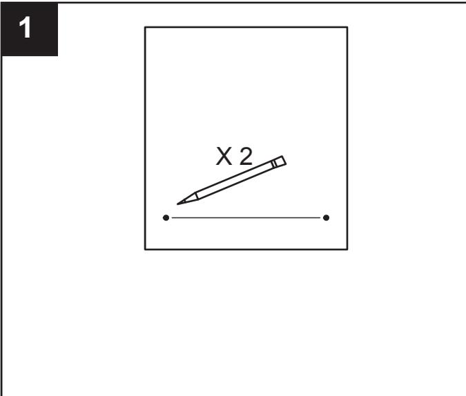
Using the template, mark screw holes. Check with level before drilling. Then, drill two 7/32" pilot holes (for masonry wall) or drill two 3/32" pilot holes (for wood wall, no anchors needed).
