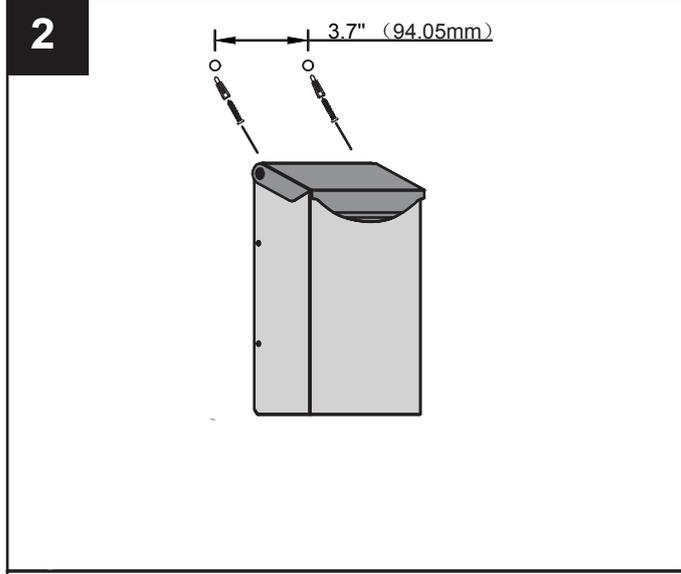
For brick or other masonry walls, insert the anchor into the wall. Install screws, ensuring to leave a gap of 1/4" between wall and screw head. Anchors are not needed for a wood wall.
