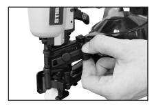
•Depress the latch on the Nail Gate and Basket Cover. Open the Nail Gate and Basket Cover. Place one nail coil in the Basket so it fits securely around the center post.
