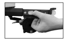
• Slide caps along the Feed Chute with fingers until the first cap is positioned under the Nose.
