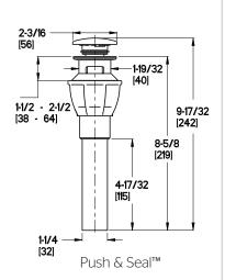
Ø1 Min to Ø1-1/2 Max. Deck Hole Openings
