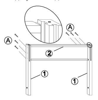
**Step 2** The other side of (1), insert each (3). Align and screw in (A).
