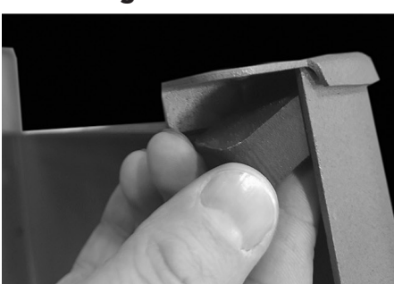
Figure 5 – Right Door Cap seal Installation
