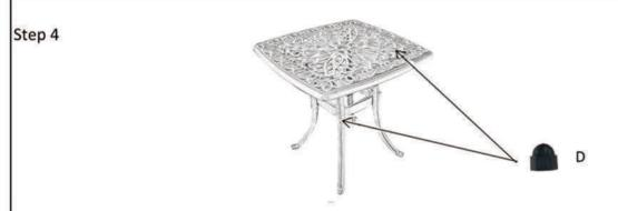
Tighten all Nuts with Wrench.And Turn over the table.Adjust the pre-installed Rubber Pad (L) until the Table is level with the ground ,Tighten all the nuts and cover them with nut caps(D).Your table can use now.
