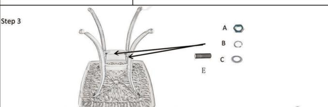
Attach the Stud M8(L) mito the realistic table leg), Then, Attach the Table legs Support (3) to the four Legs (2) using flat washer, spring washer and nuts(A,B,C)DO NOT over tighten.
