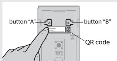
**D** If the pairing process is successful, re-name the lock in your system (if applicable).
