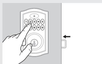
**C** Close the door. Press the "Lock" button. Confirm that the door locks smoothly without error.
