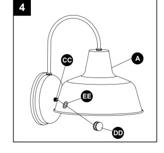
5. Install light bulb (not included). Use one 60-watt max. standard-base bulb or one 13-watt standard-base CFL bulb.
