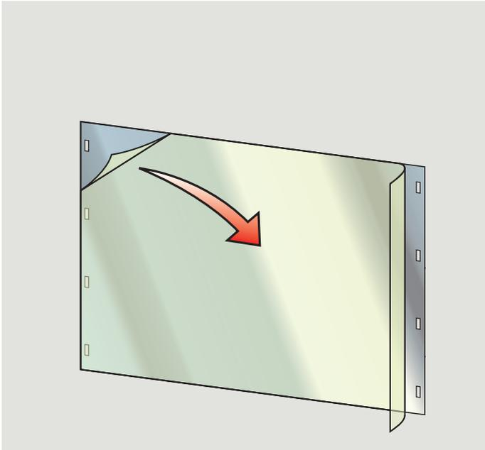
**ENGLISH:** Remove protective film from the rigid tunnel section.
