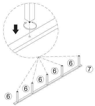
Adjust the leveling feet of the legs (6) to ensure all slats (5) are leveled and staying at the same level.
