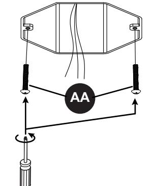
Insert the mounting screws (AA) about 1.0 inch into the Junction box
