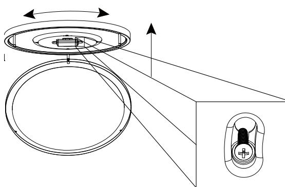
Place the fixture pan (A) over the pre-installed mounting screws and the
