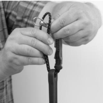
First pass the loop through the hole of the tool and pass D-ring end through the tool attachment loop forming a knot on the captive eye.
