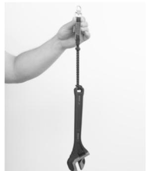
Tightly lock the knot with cord lock and the elastic tool attachment is ready to use.
