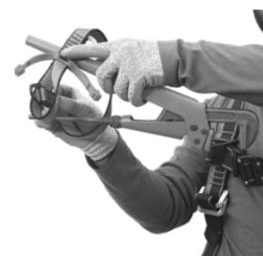
Now clinch the loop over the tool and tightly wrap the two wings of the tool attachment over the tool for strong hold grip on the tool
