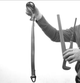
Untangle the tool attachment and pass the loop at the other end through the desired tool.
