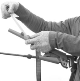
Tightly wrap the tool tape (DXDP810100) around the anchor knot for tight grip and strong stable fix of the knot on the tool.
