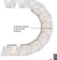
Building Curves: A radius as small as 3' can be built with 16" Basic Wall block. The bond pa ern of convex & concave curves will adjust sideways. If a stack bond situa on occurs, remove the rear lip as shown or cut units to return back to running bond pa ern.
