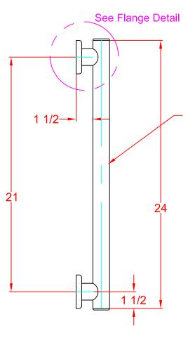
1-1/4" x 18ga. S.S. Round Tubing formed to eliptical shape of 1-1/2" x 1"
